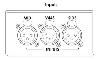
**V44S** - This 5-pin XLR connector connectors the V44S microphone to the splitter box. It routes to all three outputs.
