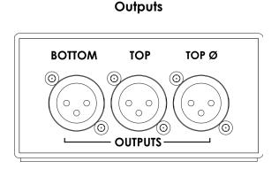
**BOTTOM -** This 3-pin XLR connector routes to the bottom capsule of the V44S microphone - or the "MID" input in the case of using two mono microphones.
